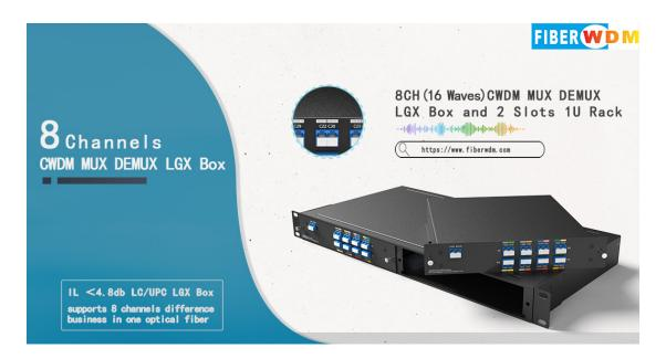
The single fiber 8channels (16 waves) CWDM MUX DEMUX is designed by FIBERWDM, A side's waves are: RX 1310nm to 1450nm/ TX 1470nm to 1610nm, and B side's waves are: RX 1470nm to 1610nm/ TX 1310nm to 1450nm; it is passive CWDM device and plug-in LGX box, can plug in 2slot 1u rack, support 8channels difference business in one optical fiber for bi-direction point-to-point transmission.
